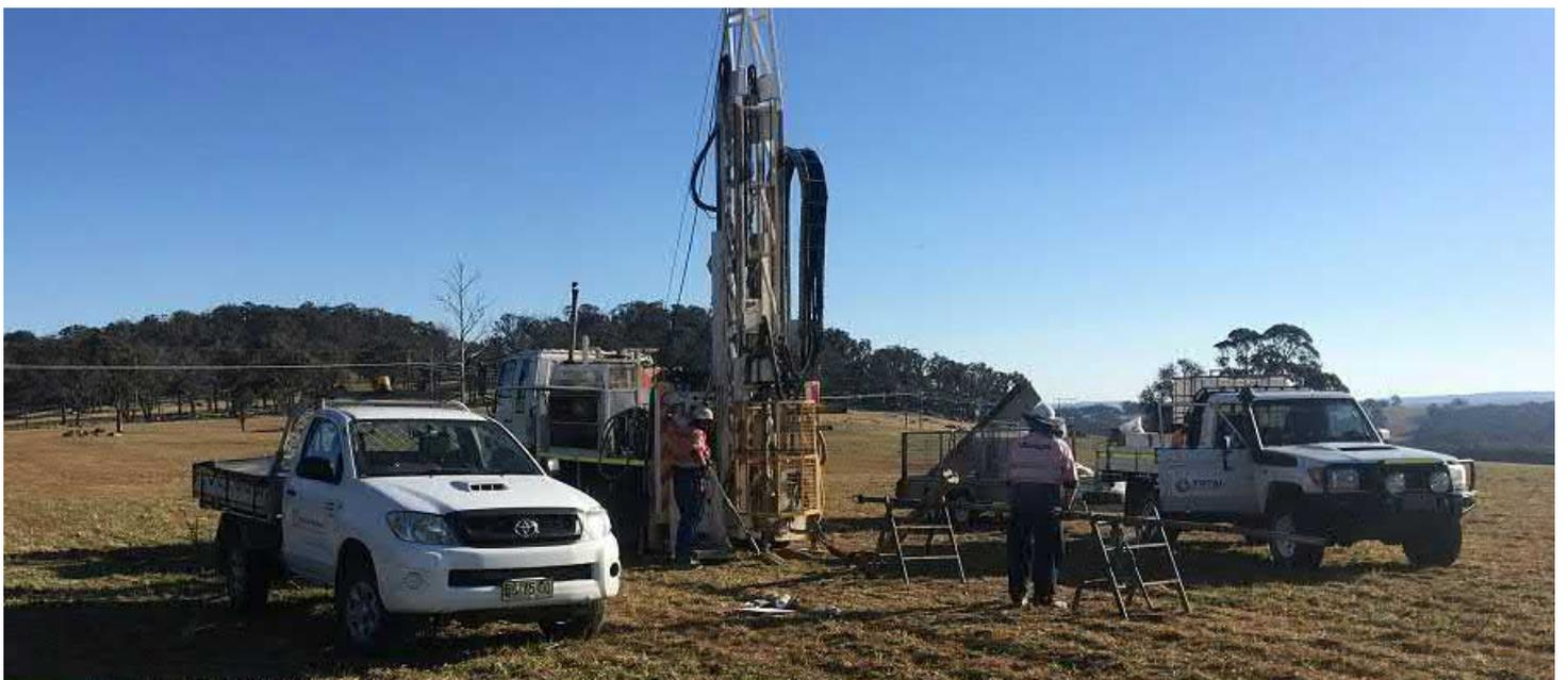
Fig 3: Typical setup for a geotechnical investigation
